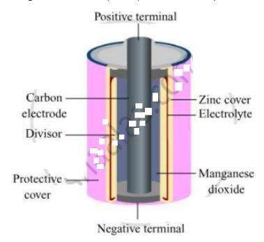
**Working of dry cell:** Chemical reactions take place between the electrolyte, zinc container and graphide rod. Because of this, electric charge is produced on the two terminals of the cell and electric current flows in the circuit.
